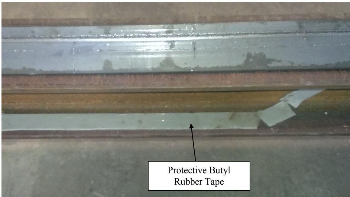
**Figure 3.2 - Protected FBG Fiber on Steel Beam**
