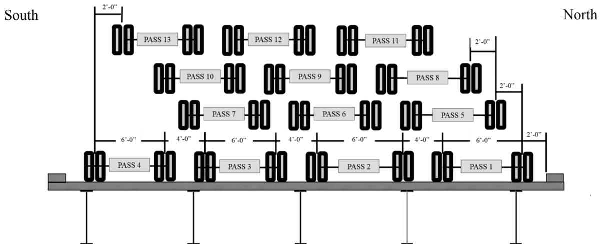
**Figure 6.4 – Vehicle Load Test Plan**
