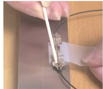
5. Cure Epoxy: Plate a metal plate over the os3120 and secure by taping. Clamp the plate to the surface. Allow epoxy to cure at room temperature for approximately six hours.
