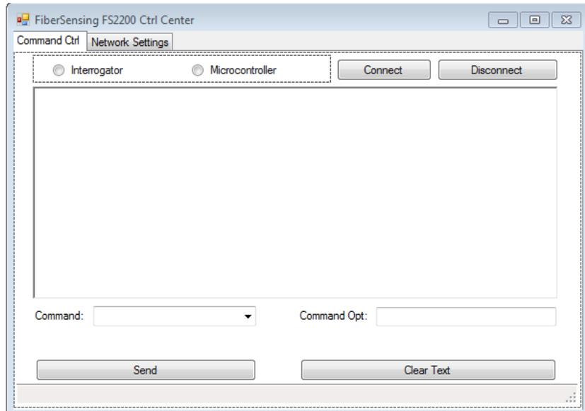
**Figure 5.15: Window display for controlling the FS2200 interrogator**
