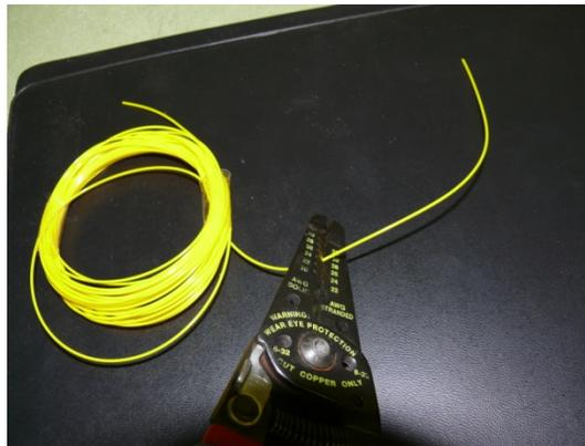
**Figure 1.3: Stripping outer coating of optical fiber.**
