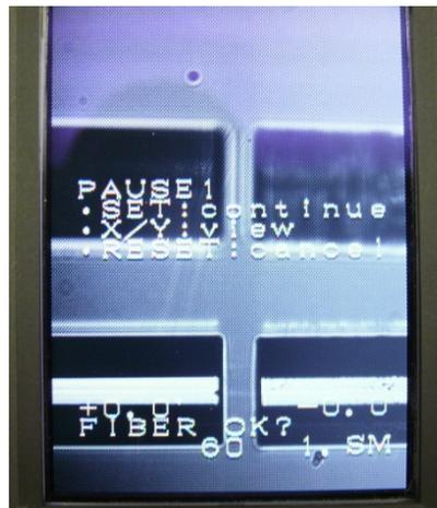
**Figure 1.9: Well-Prepared Fibers**
