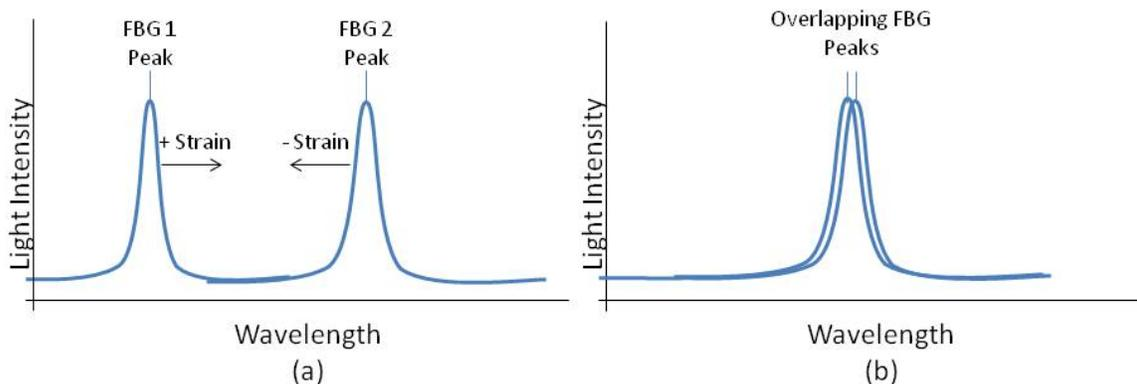
**Figure 3.1 - Interrogation Overlap Due to Inadequate Sensor Spacing**
